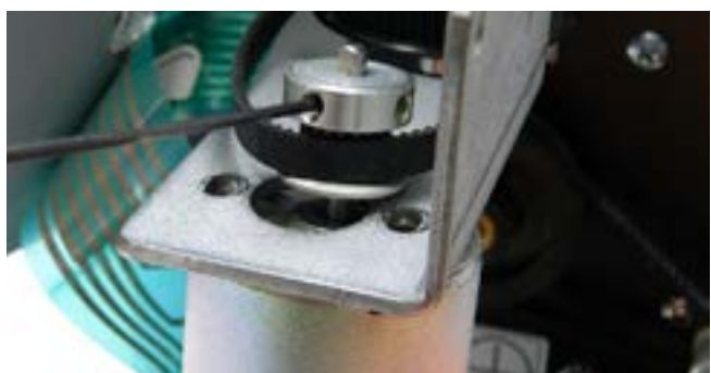
Step 16: Slightly tighten the set screw onto the flat part of the shaft. No need to fully tighten at this time.
