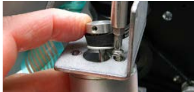
Step 11: Remove all 3 screws from the motor while holding on to the pulley as shown. Slide the motor down from the shaft and place on the table.
