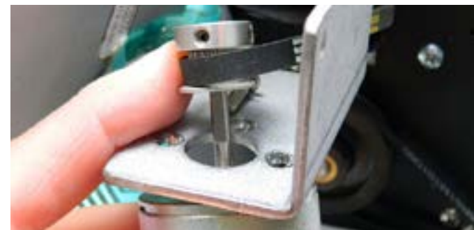
Step 15: Slide the Y pulley onto the shaft of the motor that was taken from the inside of the CPII (X motor) as shown.
