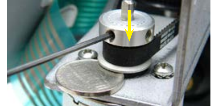
Step 18: With the motor screws (3) slightly tighten, and the nickle in place, press down on the pulley (arrow) until the pulley touches the base as shown. You can now fully tighten (clockwise) the 1st set screw.
