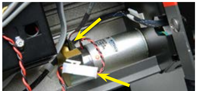
Step 8: Unclip both the white (power) and the black (communication) connectors (red arrows). You can now pull the X motor (with the pulley still attached) away from the end plate. NOTE: You will be removing the pulley soon.
