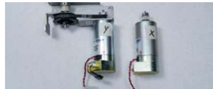
Step 13: Both motors and pulleys are marked. IMPORTANT: Even though the motors are the same, THE PULLEYS ARE NOT THE SAME. The Y PULLEY MUST stay with the motor that you are switching and placing on the Y transmission.
