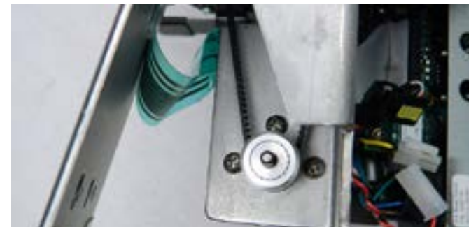
Step 21: This view shows how the pulley, the 3 screws and the Y belt should appear.
