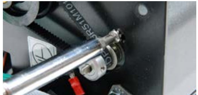
Step 6: Remove the 3 screws that secure the X motor to the end plate.
