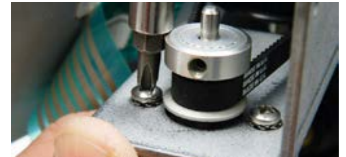
Step 20: You now must tighten the small Y belt. To do this, (with all 3 screws not fully tightened yet), wrap your fingers around the motor and your thumb against the bracket as shown, pull the motor towards you until the belt is taught. Now tighten all 3 screws.
