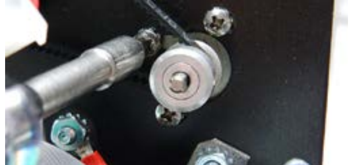
Step 26: Place the Y belt around the motor pulley (silver) and the large black plastic pulley. Place the 3 screws through the end plate and into the motor as shown. Don't tighten at this point. You still need to pull the motor tight to increase the tension of the belt.
