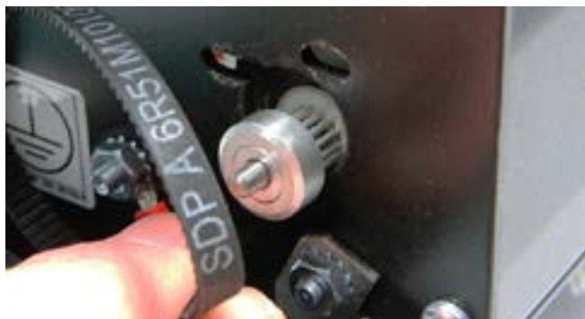
Step 7: With the 3 screws removed, the X motor is loose enough to remove the X belt as shown. NOTE: Leave the X belt as shown. No need to remove it totally.
