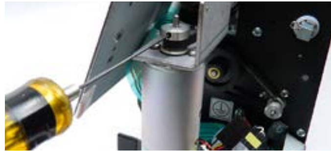
Step 10: With the 1/16" Allen wrench, unscrew (counter clockwise) both of the set screws on the pulley. NOTE: Do NOT unscrew the set screws all the way, 1 full turn should suffice. The pulley will NOT slip through the hole in the bracket.
