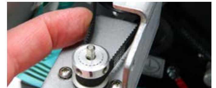
Step 22: To test the tension of the belt, press in on the belt at this location. It should not press in more than 1/8th of an inch.
