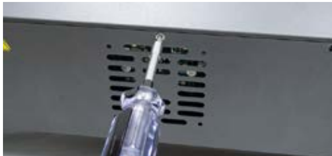
Step 5: With the CPII still tilted back, remove all 7 screws that hold the bottom cover. Remove the bottom cover from the machine and place to the side. This will expose the X motor.
