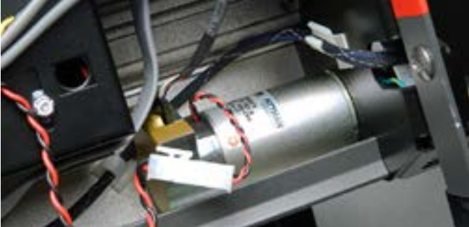
Step 25: Place the X motor in the CPIO as shown. The pulley will slide into the opening. You can, at this time, re-connect both the power and the communication clips.
