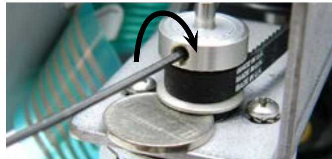
Step 19: Turn the pulley until you have the 2nd set screw in view. You can now tighten (clockwise) the 2nd set screw.
