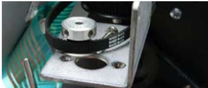
Step 12: The pulley that is shown is from the Y motor. This pulley must stay with the Y transmission bracket. IMPORTANT: To avoid confusion, mark the pulley and the motor with an X. See step 13.
