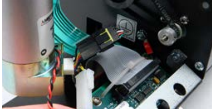
Step 9: Before removing the Y motor, disconnect both the communication (white) and the power (black) connectors.
