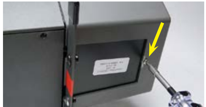
Step 4: With the CPII tilted, remove the silver screw (arrow). You can now remove the cover to expose the Y motor
