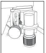
5. Rotate the clamp back down and tighten the thumbscrew until the blade holder is secure.
