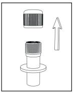
Insert the blade into the blade holder and push the blade into the blade holder until it 'CLICKS'. Screw the cap back onto the blade holder.
