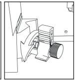
4. Insert the blade holder making sure you put the enlarged disk into the slot on the carriage.
