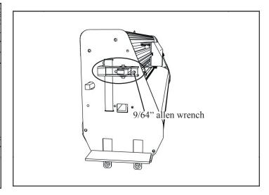
5. Remove the cover of the carriage by removing the two cover screws.
