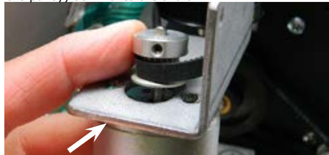
Step 15: With the Y motor placed up tight against the bracket (arrow), screw in in the 3 black screws. Tighten the screws so the motor does not move up or down. NOTE: You will fully tighten the 3 screws later.
