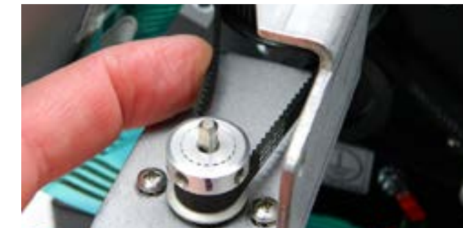
Step 21: To double check the tension of the belt, press against the belt as shown. It should press in no more than shown about 1/8th".
