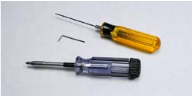
Step 1: Tools needed: 1/16" Allen Hex (L shaped or straight with handle) and a Phillips screwdriver.
