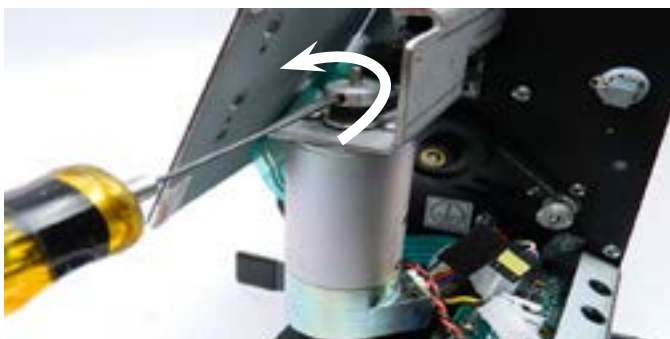
Step 7: With the 1/16" Allen Hex wrench, unscrew (counter clockwise) both of the set screws on the pulley. NOTE: Do NOT unscrew all the way. Just 1 full turn on each set screw should suffice.
