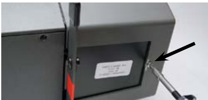
Step 3: Tilt the CPII on its back and remove the silver screw (arrow). Tilt back back on its feet.
