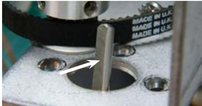
Step 12: A close up of the shaft that the pulley will slide over. NOTICE the flat side of the shaft. 1 of the set screws will be tightened against this side.
