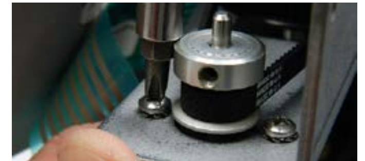
Step 20: The 3 screws are not tightened all the way at this time. With your free hand you need to pull the Y motor tight. Your 4 fingers wrapped around the motor, and thumb pressed against the bracket edge, begin to pull tight. This will cause the belt to be at the correct tension. While still holding the motor, tighten all 3 screws.
