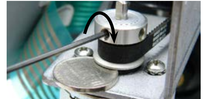
Step 18: With the 2 set screw loosened, press down on the pulley until it presses against the nickel. This will give the the correct distance. You can now tighten the set screw (clockwise) that lies against the flat of the shaft.
