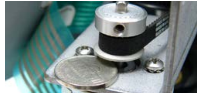
Step 17: To get the correct distance that the pulley needs to be from the bracket, a nickel can be used as shown. NOTE: The 3 screws are tightened to the point in which the motor is up against the bracket. NOTE: The spacing is .090 (2.3 metric). The nickle can be used to get a close proximity.
