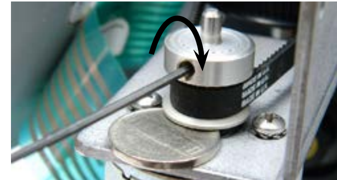
Step 19: Turn the shaft and tighten the 2nd set screw (clockwise). You can now remove the nickel.
