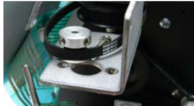
Step 10: You are now able to pull the motor down while leaving the pulley on the top of the bracket as shown.
