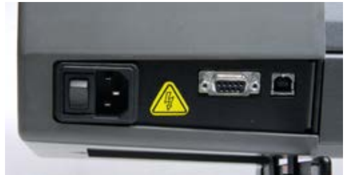
Step 2: Turn off the power and unplug the power cord and the communication cable.
