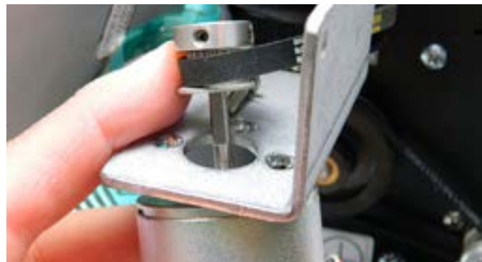
Step 13: While holding new motor with one hand, slide the pulley (with the Y belt wrapped around the teeth of the pulley) down onto the shaft.
