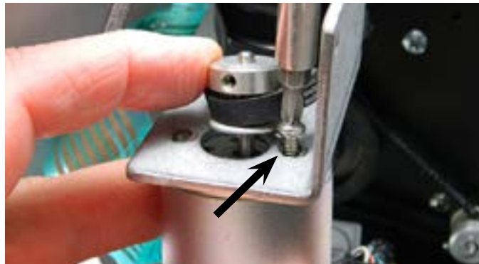
Step 9: While holding the motor with one hand, go ahead and remove the 3rd screw from the motor.
