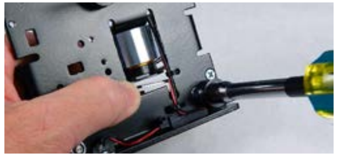
Step 26: Now you can place the nut and tighten with the 11/32" socket wrench. IMPORTANT: Do NOT over tighten this nut. When properly adjusted, the wheel rotates freely & smoothly. It does NOT move in/out on its shaft.
