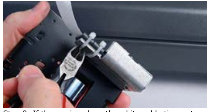
Step 8: If the carriage has the white cable ties, cut both of them with the wire cutters and discard.
