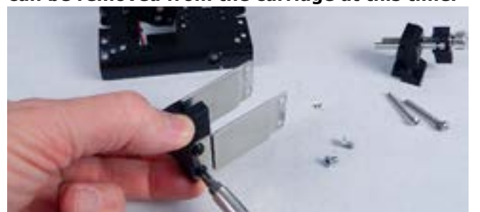
Step 14: Remove the (2) bottom black screws to release the bottom flexure.
