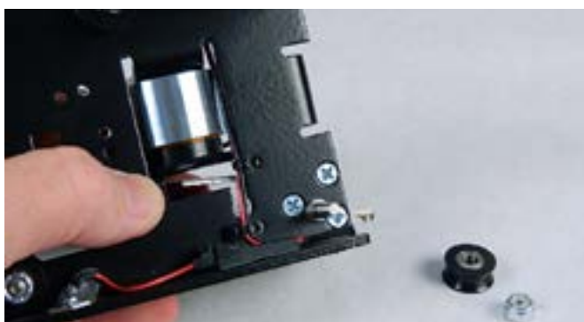
Step 23: While holding the flexure unit against the plate on the other side, insert the 3 silver screws and tighten firmly as shown.
