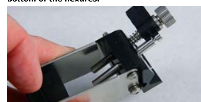
Step 20: Shown are both silver screws pushed into the jaw. NOTE: 2 washers are only on the bottom screw. You are now ready to place the unit against the carriage plate.
