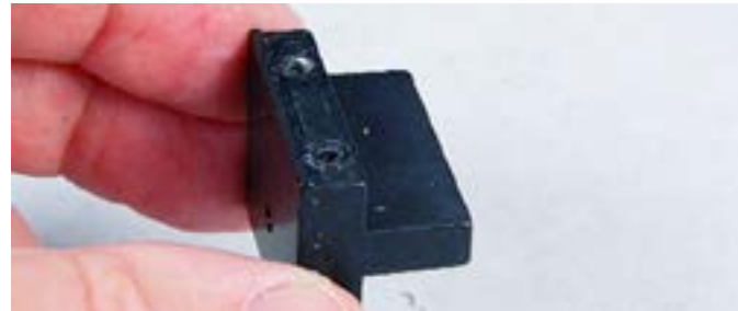
Step 16: This shows the black 'Flexure Block' that will hold the new flexures that you received. (Including all the new screws that will be needed). IMPORTANT: The 3 screw holes (Not shown) are in the back of this block. They will face the carriage plate.
