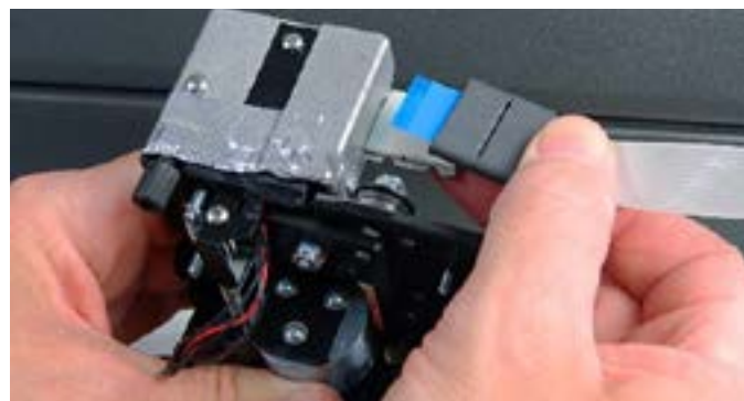
Step 9: After the cable ties are removed, you can pull the ribbon cable out until it releases from the carriage board as shown.
