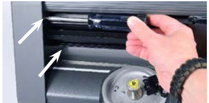
Step 4: With the Phillips screw driver, remove both the 2 screws (arrows) from the left end cover.
