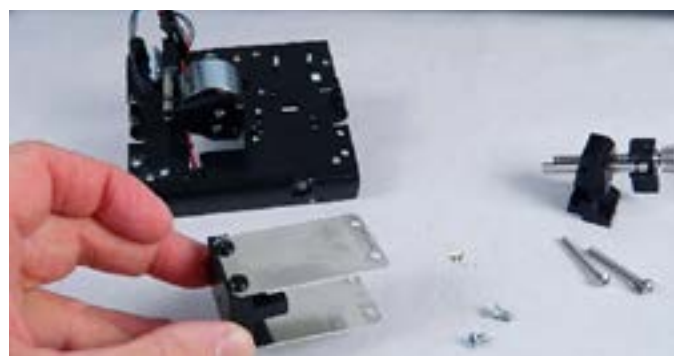
Step 13: The flexure mechanism is ready for the next step of the removal of the (4) black screws.
