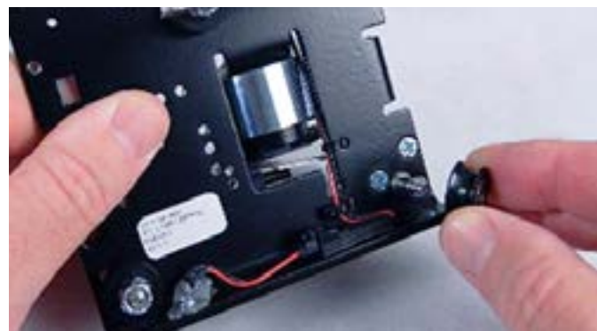
Step 10: Remove the nut from the wheel with the 11/32 socket wrench then slide off the wheel. This will expose the 3 screws that will need to be removed.
