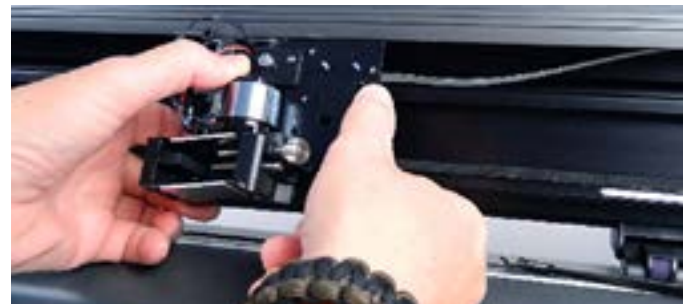
Step 28: Re-place the carriage back on the traverse. Top wheel first, press down, then push the bottom of the carriage in so the 2 bottom wheels rest on the bottom of the traverse. The carriage should move smoothly.
