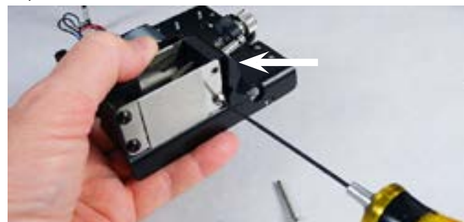
Step 12: With the 5/64 allen wrench (The smaller of the 2 allen wrenches), remove both (2) of the silver screws from the bottom flexure as shown. This is the point that the flexure mechanism can be removed. NOTE: The flexure mechanism and the black jaw can be removed from the carriage at this time.
