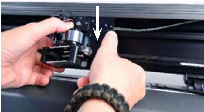
Step 7: Remove c-stick assembly, then the carriage by pressing down, then pull out from the bottom.
