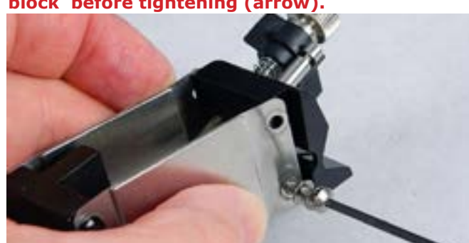
Step 19: Place the jaw (arrow) between the 2 flexures and start the one silver screw with (2) washers. You can slide these screws in (no threads in the black jaw).
