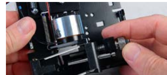
Step 24: Turn the carriage back around so the jaw faces you. IMPORTANT: Move the jaw up and down. It should be smooth and NOT rub on the coil. If it does rub, loosen the silver screws a bit, shift the jaw, then re-tighten. Have patience.
