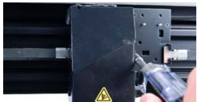
Step 32: Once the carriage has moved left to right smoothly, place the carriage back on with the (2) screws. You are ready to resume. ...FINISHED
