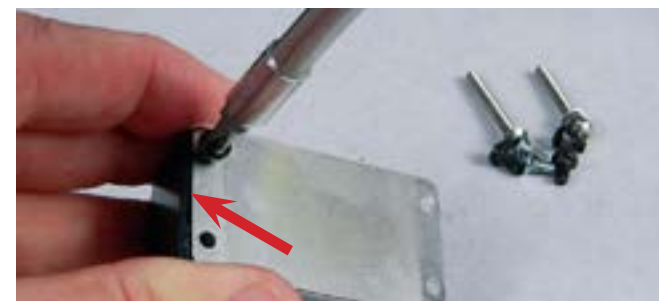
Step 17: Place the new flexure (top) on the Flexure Block and secure the (2) black screws. NOTE: The 'Stiffener' is on the bottom of both flexures. Repeat for the bottom flexure. IMPORTANT: Make sure that the flexure is seated against the lip of the flexure block before tightening (arrow).
