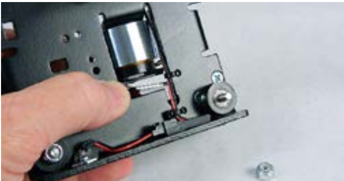
Step 25: Once the jaw and flexure unit is placed, go ahead and place the wheel over the threaded shaft as shown.
