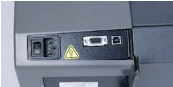
Step 3: Turn off and un-plug both the power cable and the communication cable.
