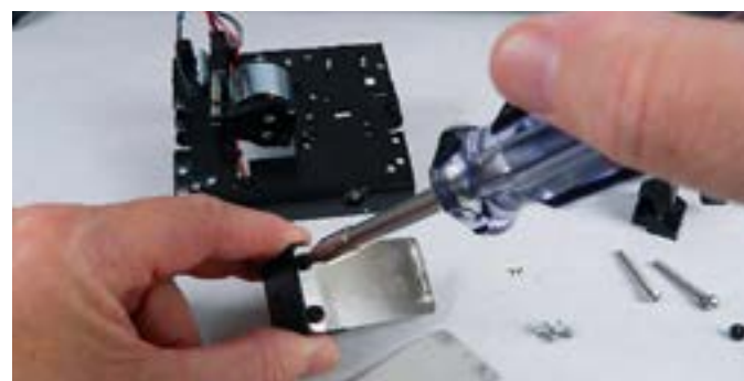
Step 15: remove the (2) top black screws from the top flexure. You can dispose of the 2 damaged/bent flexures.
