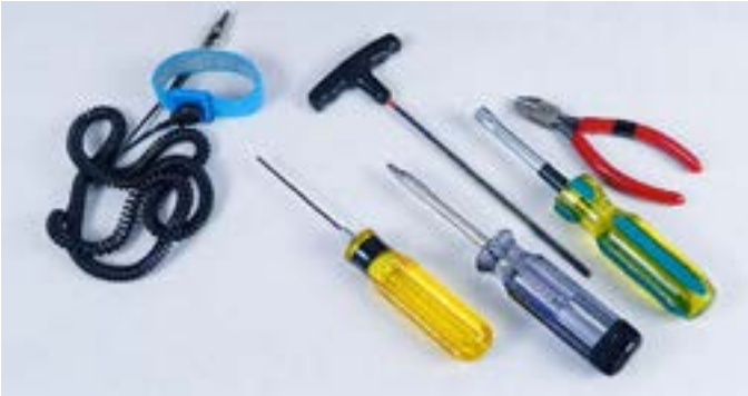
Step 1: Tools needed: Anti-static wrist strap, philips screw driver, 11/32" socket wrench, 5/64" Allen wrench, a 9/64" Allen wrench, and a wire cutter.
