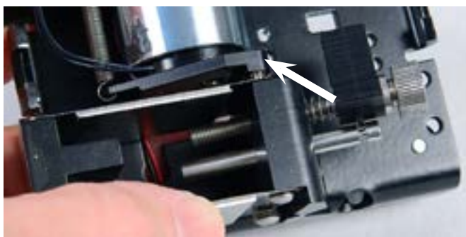
Step 21: With the flexure unit pressed flush against the carriage plate, you are ready to thread the 2 screws into the coil base plate (arrow).
