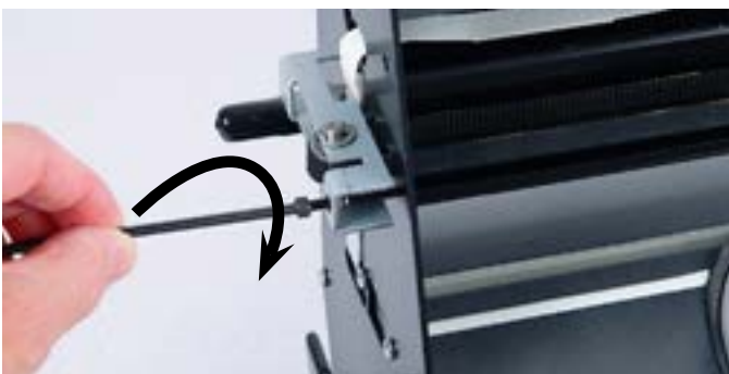
Step 31: Re-tighten the tensioner. Turn 2 full turns clock wise. Just the opposite of step # 5.
