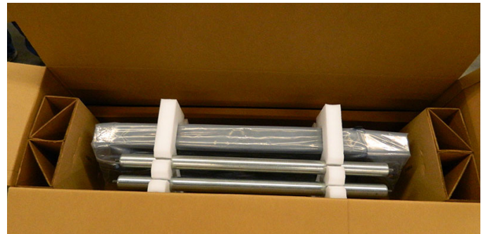
Step 10: This shows the I/S placed in the carton. The 2 metal rollers are shown. NOTE: It is NOT necessary to ship the rollers back for the repair of the machine.
