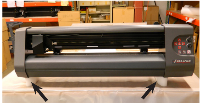
Step 2. Arrows point to the foam feet. [These must be installed to prevent damage to the bottom of the I/S 60 and to the carton].
