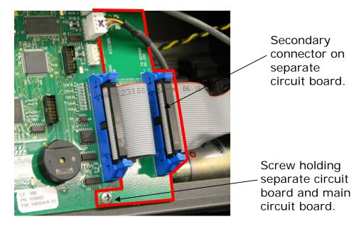
A properly installed main circuit board looks like this:
