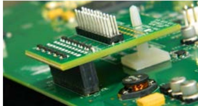
Step 14: Another angle showing how the EMI should appear. No prongs seen, and the stabilizer with the adhesive pressed onto the board.
