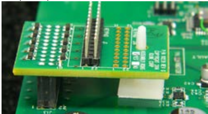
Step 13: This photo shows the EMI board correctly pressed down upon the main board.
