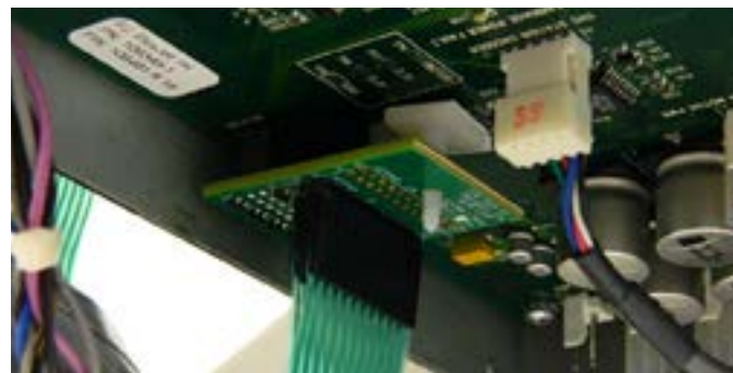
Step 16: Shown is how the EMI and the keypad cable should appear.
