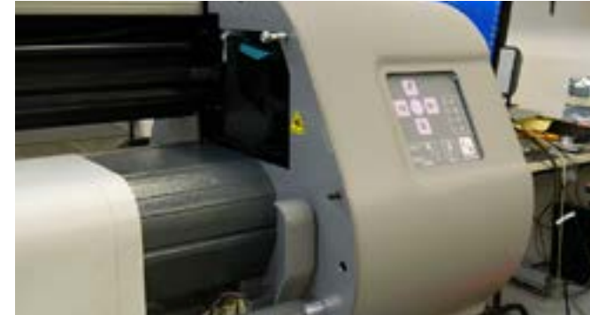
Step 21: Plug back in the power chord and communication cable. You are ready to resume printing. ...FINISHED
