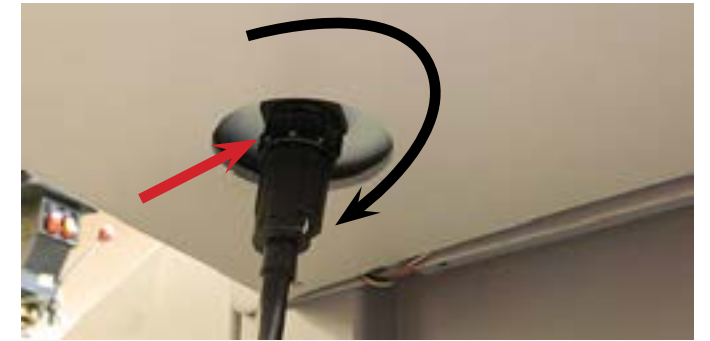
Step 20: You must re-attach the take-up motor cable. Turn the knurled ring clockwise to tighten.
