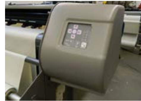
Step 19: Place back on the right end cover and attach with the same 5 screws as before (step 3).
