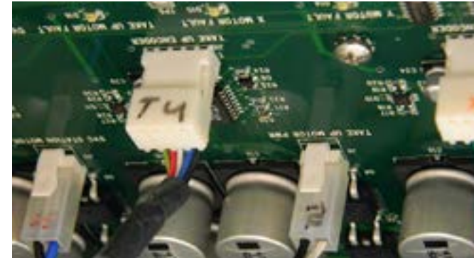
Step 17: While holding the metal cover in one hand, you need to re-attach the 2 white connectors, the take-up encoder and the take-up motor as shown.
