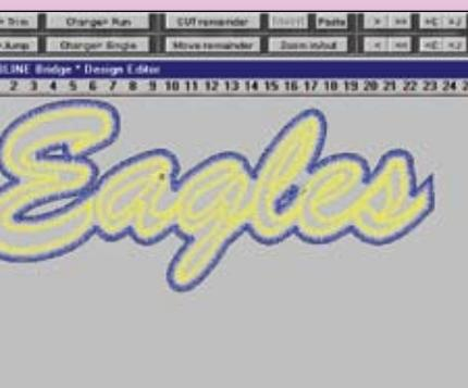
Modify stitches? Use the 301 Software to get color change codes, move stitch-start jumps to trims, or add and delete stitches. Select your desired embroidery format (.ajima .DST, Melco .EXP, etc.) and the software automatically creates a sew disk.
