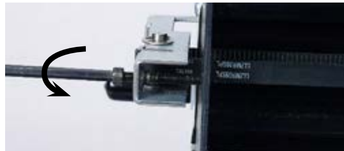
Step 16: Once both ends of the Y belt are attached to the carriage base plate, NOTE: Make sure that the tensioner is placed in the the (3) indents on the end plate. turn the tensioner set screw with the 9/64" allen wrench 2 full turns clockwise to re-tighten.
