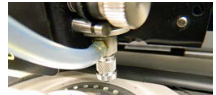
Step 22: The carriage will move over the selected bowl and pick up the stone and place it on the media. You are looking for the c-stick to be centered on the stone. Once you are satisfied with the alignment with both bowls, Re-cycle the power. You are now ready to run the CPII..... FINISHED
