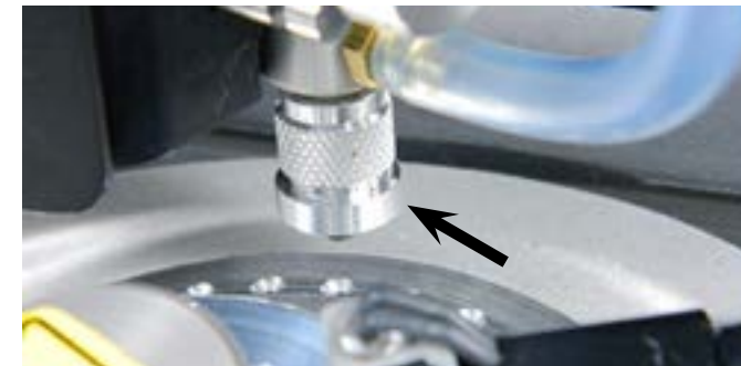
Step 21: Remove the tool tip and place the pick up tip back on (arrow). You will need to do a quick test with 6ss or 10ss stones to confirm the ideal location.
