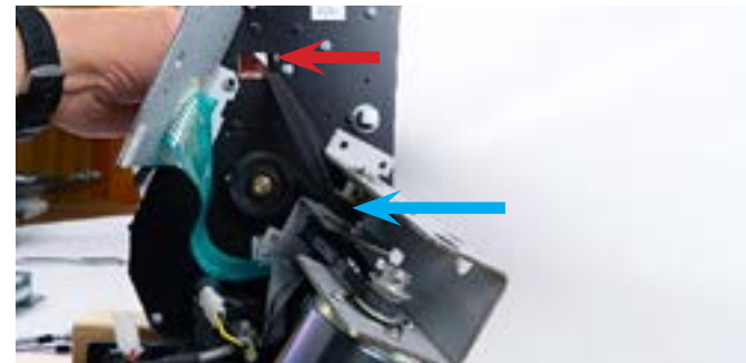
Step 11: With the new Large Y motor transmission, thread the Y belt around the top pulley (blue arrow), then through the rectangle hole in the right end plate (red arrow). NOTE: Make sure that the belt is NOT twisted.
