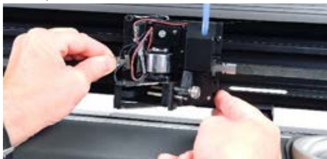
Step 15: You need to re-attach the T-shape clips to the carriage base plate as shown. NOTE: Make sure that the tensioner is upright (step 16).
