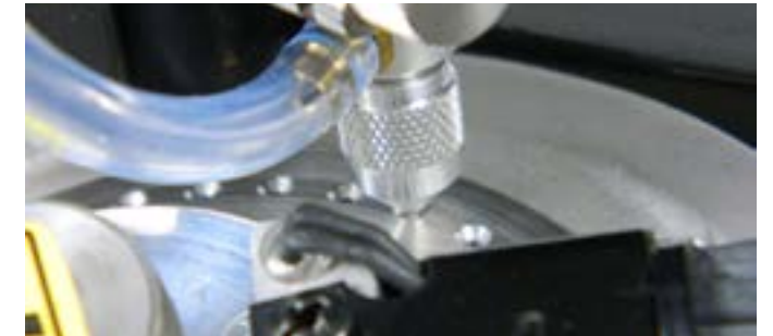
Step 20: Your goal is to have the tip fully insert into the hole in the pocket. NOTE: The procedure for aligning both bowls will guide you through all the steps.
