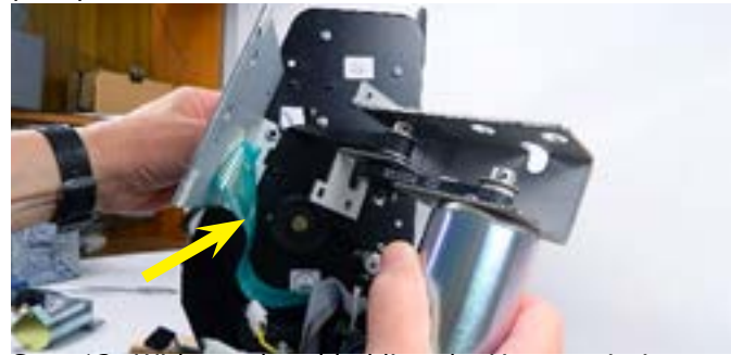
Step 12: With one hand holding the Y transmission, pull the Y belt tight with the other hand. Align and place the new Large Y motor transmission onto the 4 threaded studs. Hand thread one locking nut to hold. NOTE: You may need to move the green ribbon cable out of the way from the studs (yellow arrow).
