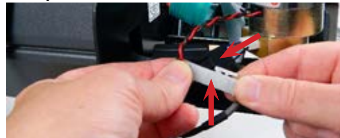
Step 14: Press the (2) white power clips together and the (2) black communication clips together (arrows). You will hear a clicking sound when successful.
