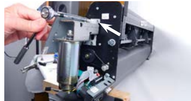
Step 13: When all (4) locking nuts have been hand threaded onto the studs, use the 11/32" socket wrench with the 6" extension and tighten all (4) locking nuts securely.
