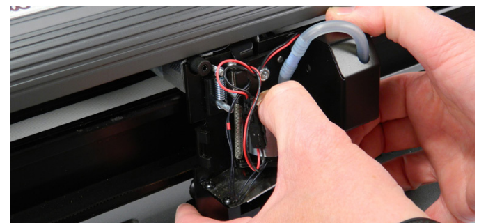
Step 24: After attaching the new ribbon cable to the carriage, place the carriage back on the traverse. NOTE: All (3) wheels should be on the traverse and the carriage should slide smoothly.
