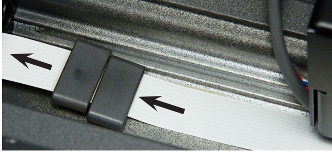
Step 17: This shows the old ribbon cable ready to pull out from the still attached ferrites. The arrow points in the direction in which the ribbon cable is pulled free from the CrystalPress.
