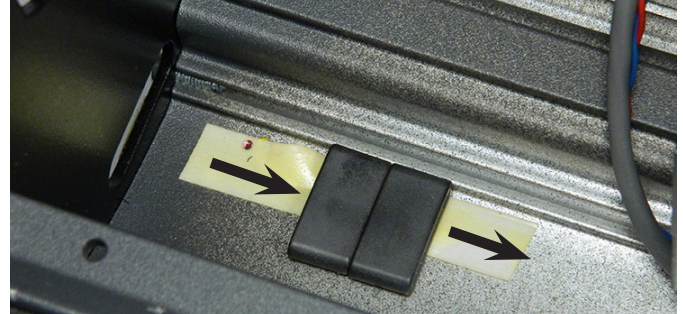
Step 18: This shows the old ribbon cable has been fully removed. The 2 ferrites remain where they are, still attached to the piece of tape. NOTE: The new ribbon cable will slide through the ferrites (step 29).
