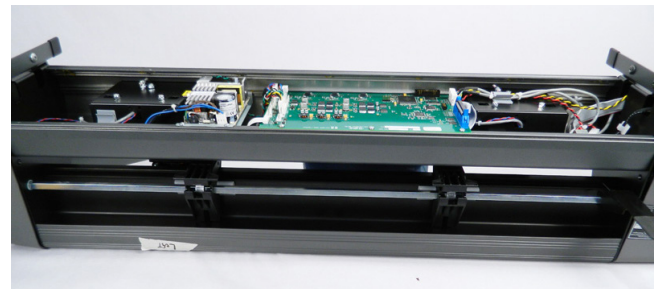
Step 14: NOTE: Will need to be supported so the CPIO does NOT roll back. The CrystalPress on its top (shown). This will give you access to the ribbon cable and main board.
