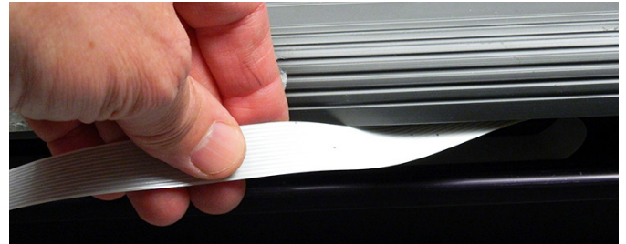
Step 10: Place the carriage on the table and pull the ribbon cable free from the 2 strips of tape that hold this ribbon cable to the inside of the traverse. The tape should stay attached to the traverse. You should be able to re-use those strips of tape for the new ribbon cable. NOTE: If the tape pulls up with the old cable, use double stick tape for the new cable.
