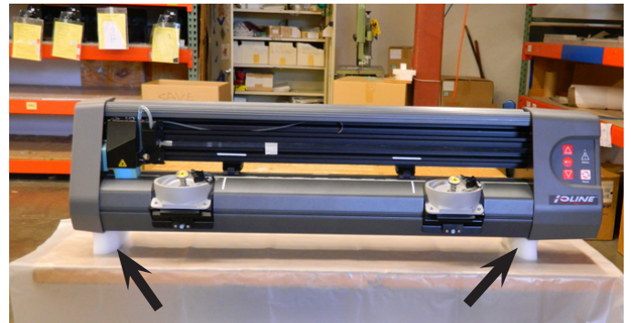
Step 2: Arrows point to the foam feet. [These must be installed to prevent damage to the bottom of the CrystalPress and to the carton]
