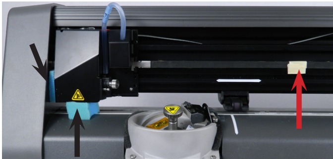
Step 3: The 2 pieces of blue foam (Black arrows) cushion and support the carriage. The masking tape (Red arrow) is wrapped around both sides of the Y belt to prevent the carriage from moving left or right.
