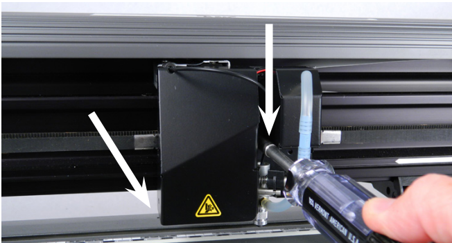
Step 29. Install the carriage cover. (2) screws. Front as shown and the left side (Arrow).
