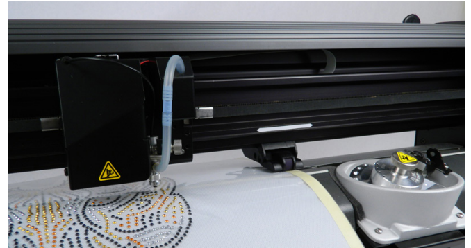
Step 30. Perform the carriage procedure to ensure the pick-up locations are correct. Contact Ioline customer support for assistance if necessary. You are now ready to print... FINISHED.
