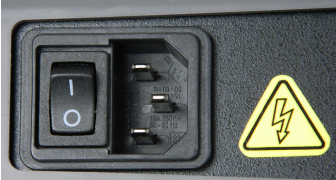
Step 1. Turn off and un-plug machine. Handling the carriage requires an anti-static wrist strap. (Included in kit)
