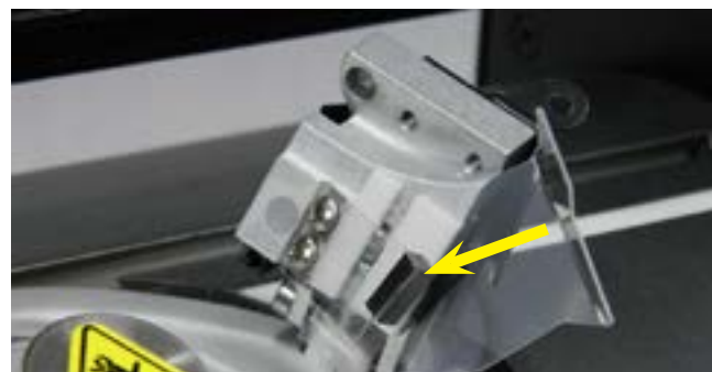
Step 8. Photo shows how the wiper (arrow) should look when affixed properly. FINISHED
