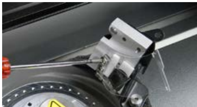
Step 4. Unscrew (2 screws) wiper and remove.
