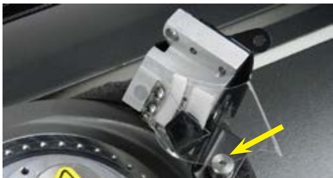
Step 3. Lift arm and use the clamp (Arrow) to hold in place.
