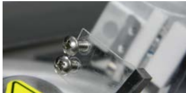
Step 6. Place the 2 screws in the wiper before you screw it to the arm. This will make it easier to attach. The wiper must be orientated as above. Foam should be facing the arm as shown
