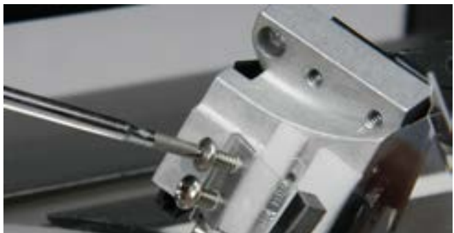
Step 7. Install the new wiper. Do NOT over tighten the screws, it could cause the wiper to fracture if tightened too much.
