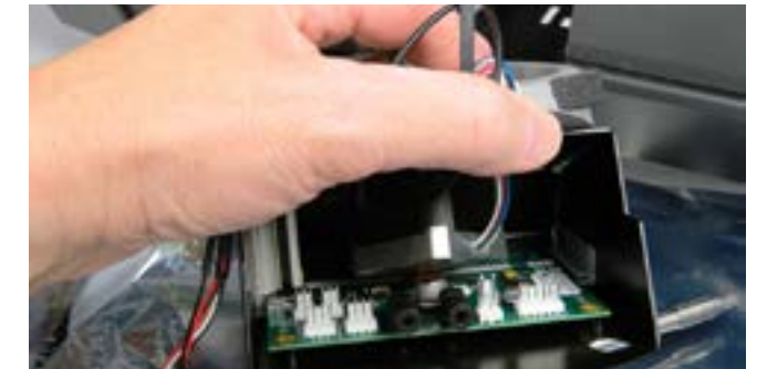
Step 20: The new board is shown placed into the clips on either side. This stabilizes the board until the 2 screws are inserted.
