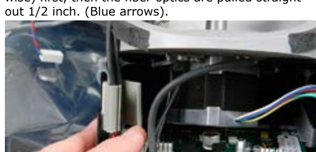
Step 14: With the clip open, you can pull out the 3 black LED wires.
