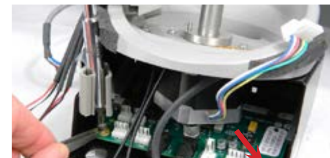
Step 21: The right side screw (Red Arrow) is inserted first. A tweezers will help to hold the screw for the left side. With the gray clip open, slide the screwdriver in the opening and tighten down the final screw.
