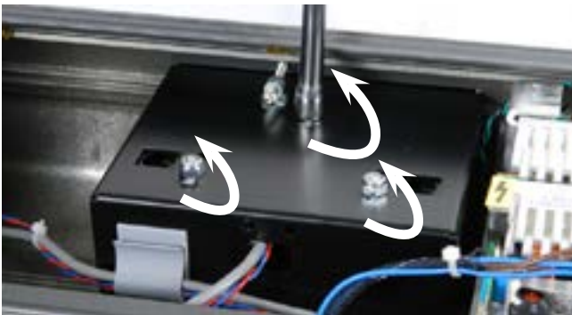
Step 3: From the sorter bowl that you need to replace the new PCB in, un-screw the 3 nylon locking nuts (counter clockwise).
