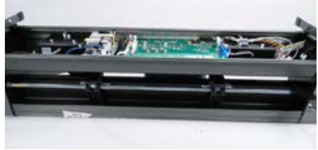
Step 2: Turn the CrystalPress over, remove the 7 screws, take the bottom pan off and place aside.
