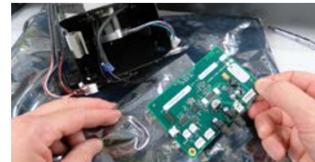
Step 19: REMINDER: The grounding wrist strap needs to be worn. The new board is ready to be inserted.
