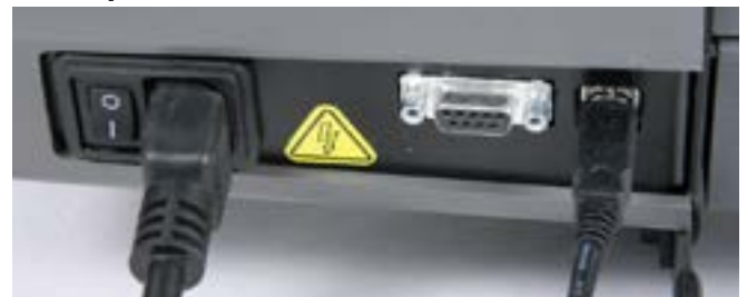
Step 32: Turn the CPII back on the legs, (No bottom cover at this time). Plug in the power and communication cords and turn on. You need to make sure that everything is connected correctly. If it is, you will need to check that the alignment of that bowl is still correct. Once you have done that, re-place the bottom cover and proceed to place stones. ..FINISHED
