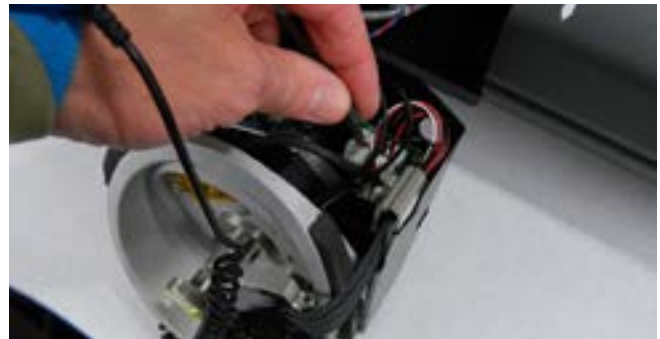
Step 26: You can turn the bowl towards the platten to attach the last 2 connections from the CPII to the bowl board.
