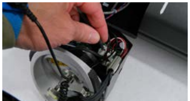
Step 8: IMPORTANT: WRIST STRAP MUST BE WORN UNTIL FINISHED WITH THE INSERTION AND CONNECTIONS ON THE BOARD.
