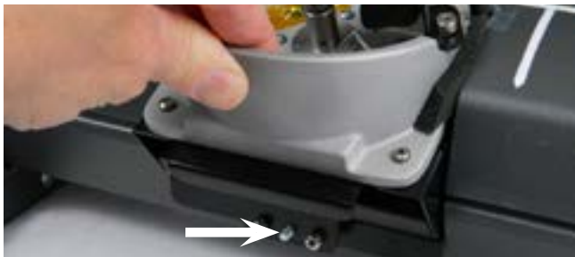
Step 29: The sorter bowl is fully inserted. The threaded insert is shown (arrow) and ready for the locking nylon nut to tighten the bowl in.
