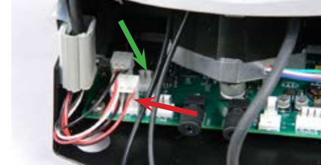
Step 23: The LED connector (red arrow) is inserted into the LED Receptor. NOTE: The receptor, (green arrow) marked 'HALL EFF' is NOT USED.
