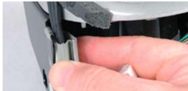
Step 13: You need to remove the black coated wires from the gray clip. You do this by squeezing the clip as shown. Index finger on the back pushing towards you, and the thumb holding in the front larger portion. This will separate the 2 locking edges.
