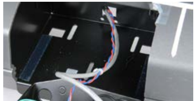
Step 28: You are ready to place the sorter bowl back into the bay bracket on the CPII. You can grab the wires and help guide them through the slot. Slide the sorter bowl into the bracket fully.
