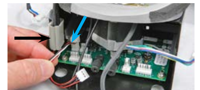
Step 22: The 3 black coated wires are placed back in the gray clip and the clip is snapped closed (black arrow). The Arm Sensor (blue arrow) is plugged into the Arm Sensor Receptor.
