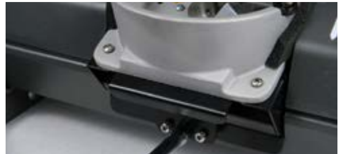
Step 30: With the 11/32" socket wrench, proceed to tighten the locking nut down until it bottoms out. NOTE: Do not over tighten, it WILL bend the metal plate in.
