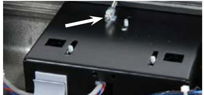
Step 4: All 3 nylon locking nuts are removed. No need to remove the silver screw (arrow).
