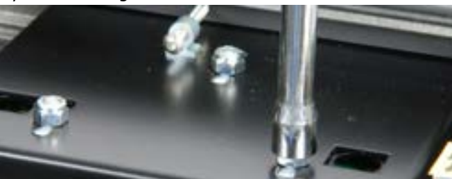
Step 31: With the CPII upside down again, you can place and tighten the 3 locking nuts. NOTE: On all 3 nuts, turn clockwise until tight, then back off 1/6th of a turn on each one. This will allow further adjustments of the bowl for the re-alignment if necessary.
