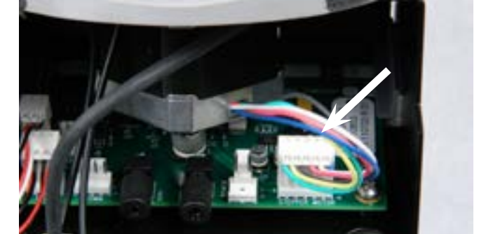
Step 24: The Stepper Motor connector has now been inserted onto the Stepper Motor receptor (white arrow).
