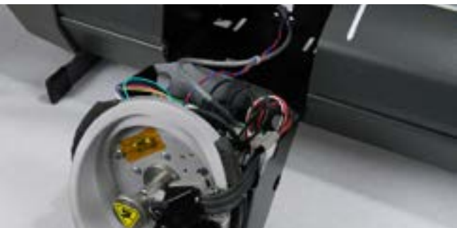
Step 7: Pull the sorter bowl towards you to clear the threaded stud, and then lift slightly up, then pull the bowl out and place it on the table as shown. (Wires are still connected to the PCB board at this point)
