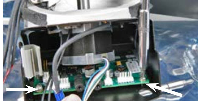
Step 16: With the Phillips screwdriver, remove the 2 screws that hold the board in. Arrows show both screws to be removed. NOTE: The screwdriver can be inserted in the clip to remove the left hand screw.
