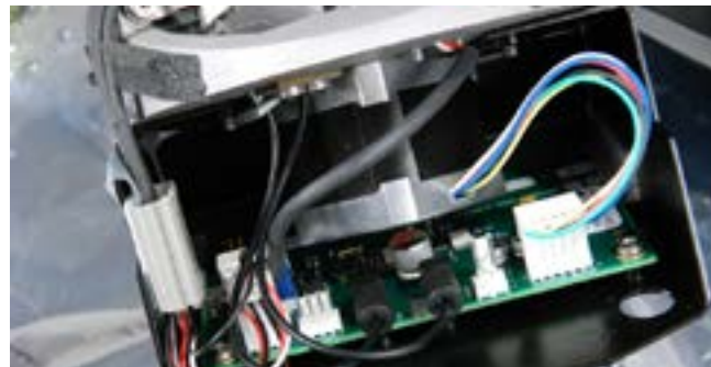
Step 11: The Sorter bowl is now free to move away from the CPIO. This will allow easier access to the remaining connectors and fiber optic cables.
