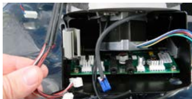
Step 15: The 3 black wires are removed, as well as all the wires. You are ready to remove the PCB board after the 2 screws are removed.
