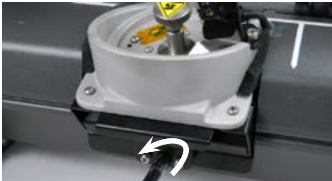
Step 5: Using the 11/32" socket wrench, un-screw (counter clockwise), the nylon locking nut from the front of the bowl as shown.
