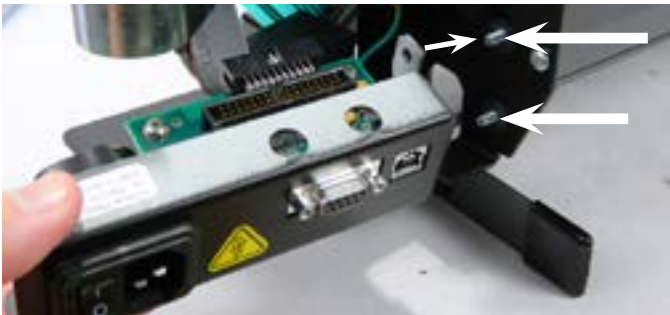
Step 27: Align the rear panel holes and slide it over the threaded studs (white arrows).
