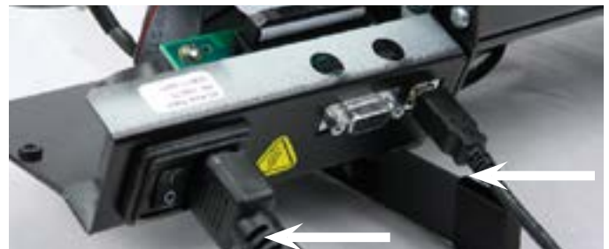
Step 32: Plug in the power cord and the communication cable and turn on to test. The carriage should move with all the lights on. A green light on the key pad will stay on when complete. ...FINISHED.
