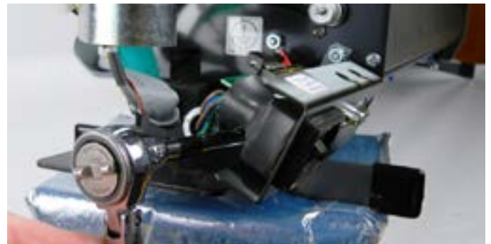
Step 8: With the 11/32" socket wrench and extension, remove the bottom locking nut. This does take some dexterity and patience.
