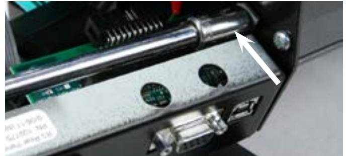
Step 28: Attach the top locking nut by hand at first to the top threaded stud, then tighten down with the socket wrench.
