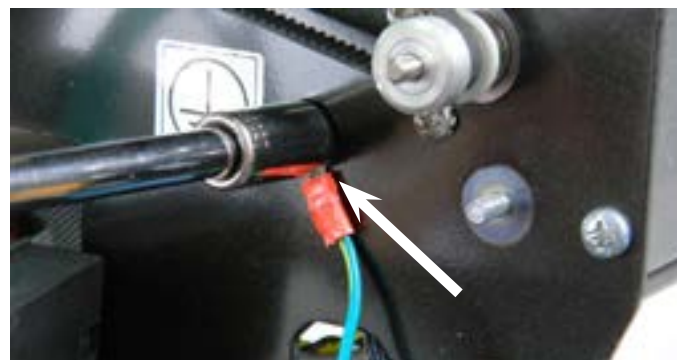
Step 10: With the 1 1/32" socket wrench, unscrew the locking nut holding the ground wire and remove the wire from the end plate.
