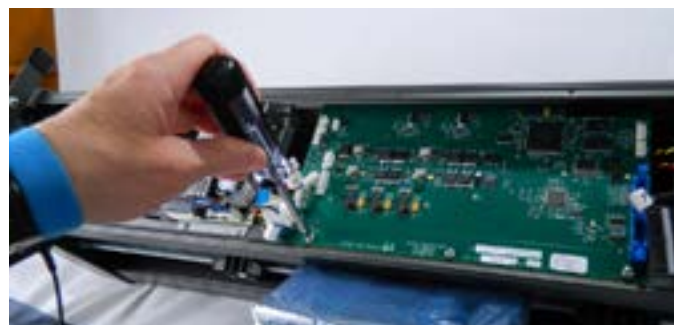
Step 15: You can now remove the (3) screws that hold the main PCB board and place to the side on an anti static bag or card board. NOTE: Anti static wrist strap is needed.
