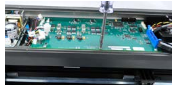
Step 24: NOTE: Wrist strap needed. Place the board back in the platen and insert the 3 screws as shown.
