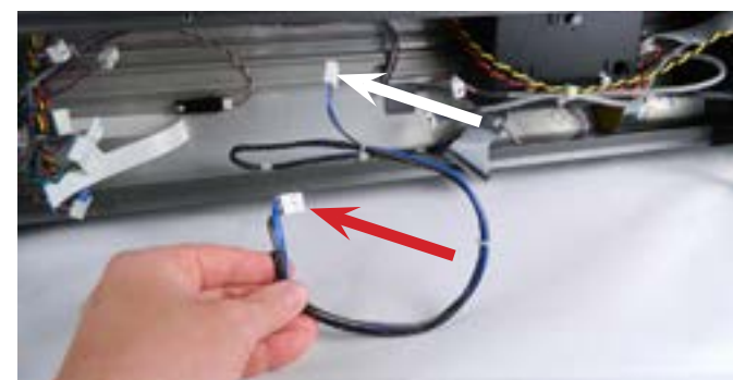
Step 21: The connector (red arrow) goes behind the power supply and out in front (Step 22). The other connector (white arrow) is not used. It is for a second power supply if added.
