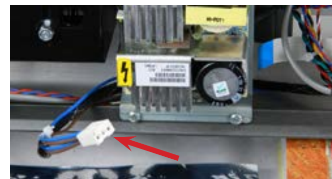
Step 22: This shows the connector wrapped behind the power supply and is ready to be plugged in. See step 23.
