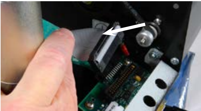
Step 5: Pull the gray ribbon communication cable up and release it from the receptor (pins).
