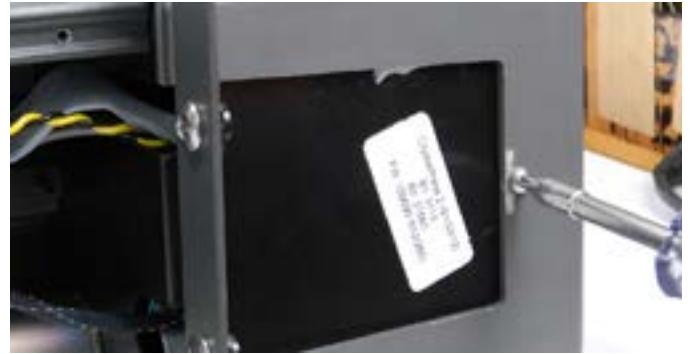
Step 2: Place the machine on its back, and remove the (1) screw on the bottom of the right cover.
