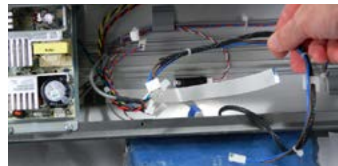
Step 17: You can now pull the black sleeved wire from under the power supply, remove the wire from the white nylon clips that are attached to the inside of the platen.
