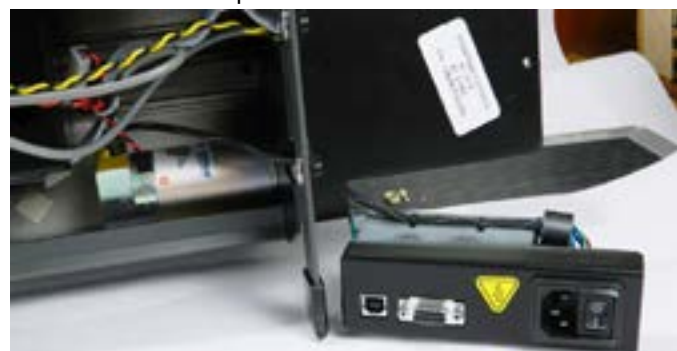
Step 12: Place the rear panel on the table. NOTE: You will need to remove the main PCB board to remove the black sleeved wire that connects to the rear panel.
