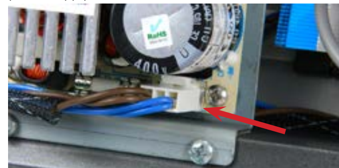
Step 23: The connector is shown plugged into the receptor on the power supply.
