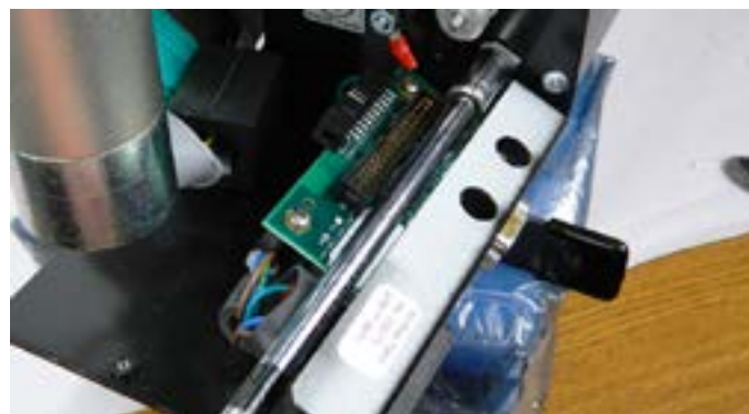
Step 9: With the same socket wrench remove the upper locking nut.
