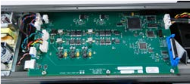
Step 25: Insert all (9) white connectors and the (2) ribbon cables back into the board. Place the bottom pan back on and secure with all 7 screws. Turn the machine back on its feet.
