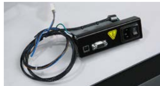
Step 19: You are now ready to attach the new rear panel.
