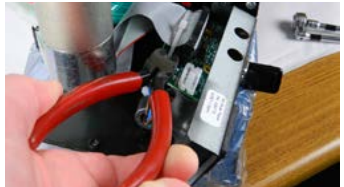
Step 4: With wire clippers, cut the cable tie so the ribbon cable can be pulled out.
