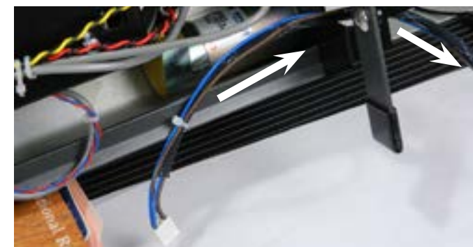
Step 18: Continue to pull the wire through the hole in the right end plate until it clears. You can place the old rear panel aside.
