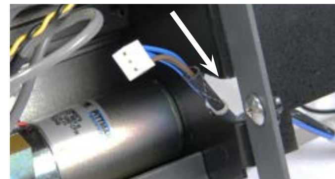
Step 20: The white arrow points to the slot in which the power cable passes through.
