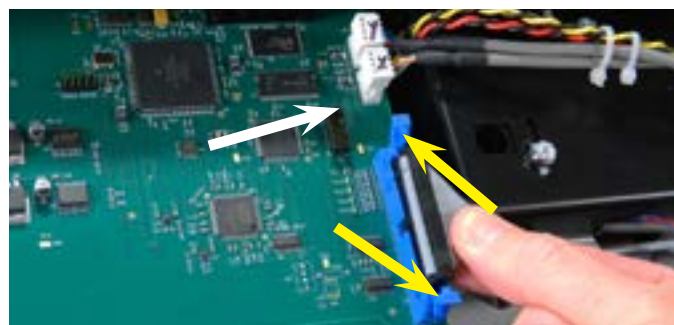
Step 13: You need to remove the X and Y connectors and the communication cable from the main board. Pull blue tabs away from middle of connector to loosen (yellow arrows). NOTE: It will help if you label the X and Y before you remove them.
