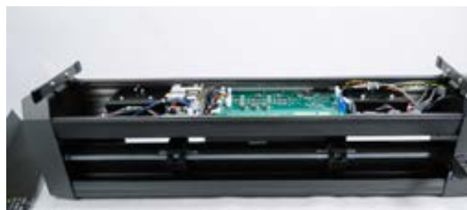
Step 11: Turn the CPII over (needs support to hold the machine stable), remove all (7) screws from the bottom pan and place the cover aside. NOTE: You can lean the CPII on its side.
