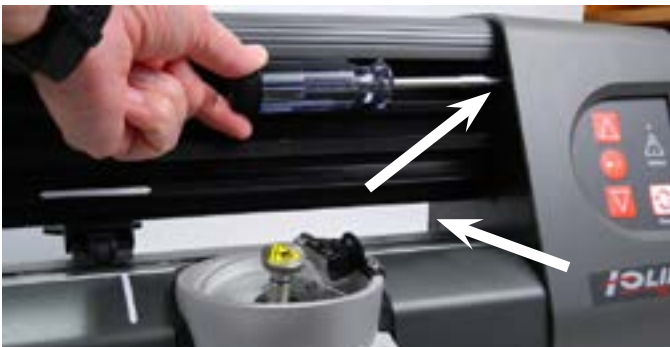
Step 3: Place the machine right-side-up. Remove the (2) screws and slide the right end cover off by pulling straight out.
