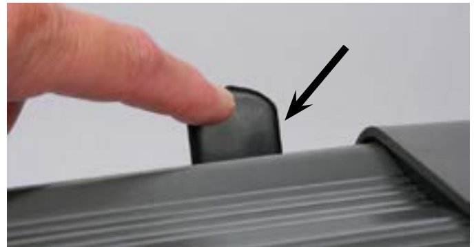
Step 2: Push the pinch wheel arm down before you turn over the machine. You will need some type of support to stabilize the up-side down machine in step 3.
