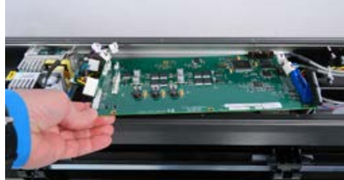
Step 16: Slide the main board into the slot in the back of the platen. The screw holes in the board align with the screw holes in the platen.
