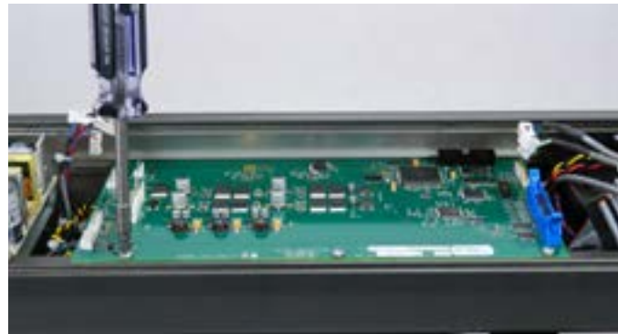
Step 13: Remove the (3) screws and slide the old board out and place to the side. You can use the anti static bag from the new board later.
