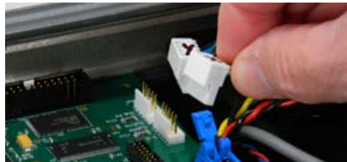
NOTE: Writing the letters X and Y on the connectors helps when re-attaching to the X and Y axis.
