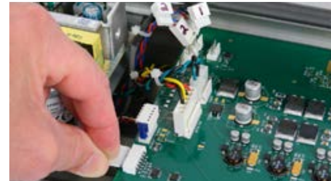
Step 23: Insert the carriage ribbon cable (silver color up) into the carriage receptor. NOTE: Push the cable all the way in.
