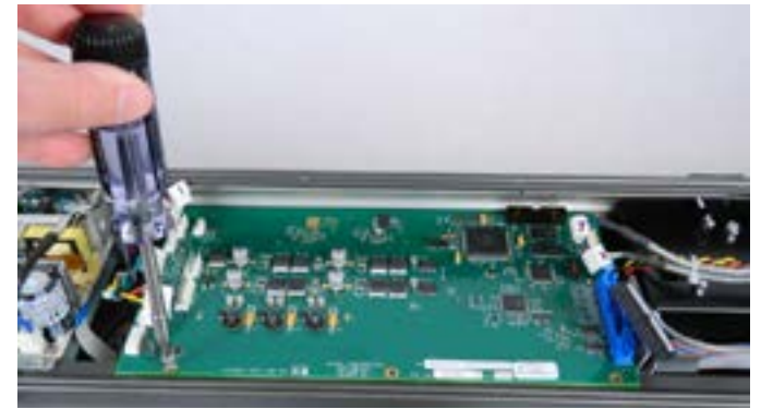
Step 18: Install the 3 screws before attaching the connectors. This will give you a stable board in which to work.
