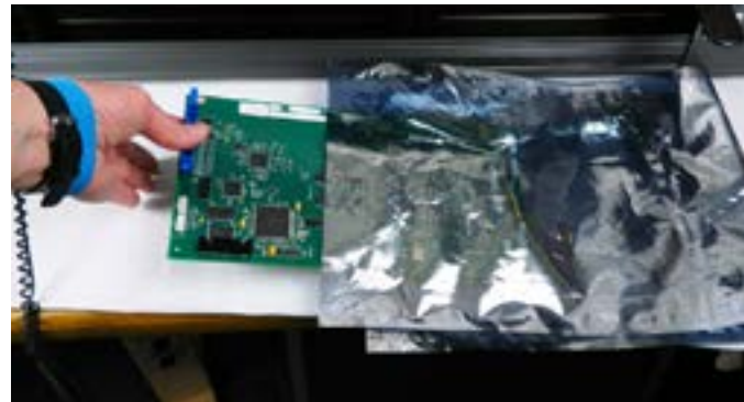
Step 14: Remove the new board. NOTE: Wrist strap is extremely important when handling the main board and any other electronics.
