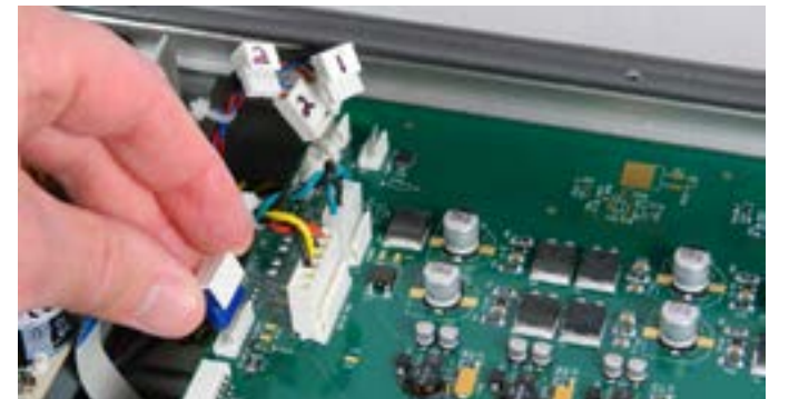
Step 22: Plug in the sensor connector to the sensor receptor pins. Push all the way down.
