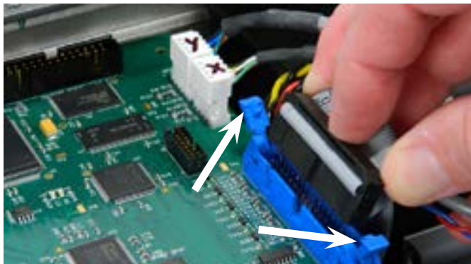
Step 27: The ribbon communication cable is being plugged in its receptor. This can only be plugged in when the blue locking (arrows) arms are in the open position.
