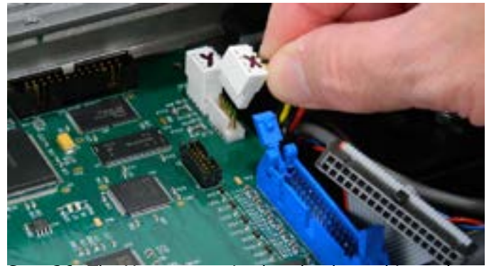
Step 26: The Y connector is already plugged in to the correct receptor (Y). The X connector is being plugged in to the X receptor.
