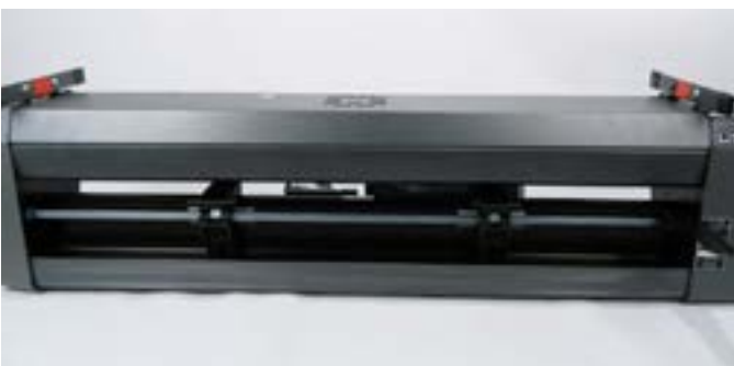
Step 31: Turn off and un-plug. Turn the CII back on its top, then place the bottom pan back on and attach with the 7 screws and tighten securely. ...FINISHED
