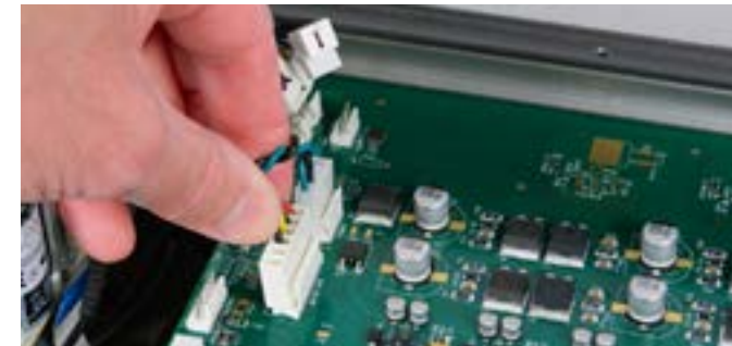
Step 21: Plug in the 'Motor Power' and the 'Power' connectors to the 'Motor Power' and 'Power' pins. NOTE: The connectors must be oriented in the correct way and pressed all the way down.
