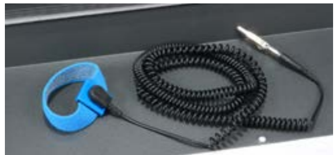
Step 4: IMPORTANT: The wrist strap is needed when handling all electronics. The blue elastic band goes around the wrist, the metal clip is attached to a NON-painted piece of metal on the machine itself.
