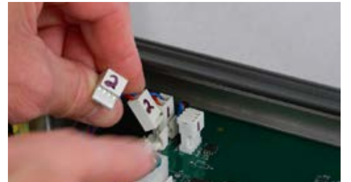
Step 24: Plug in the (2) sorter bowl and (2) sorter communication connectors to the corresponding pin receptors on the board.
