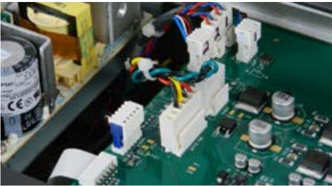
Step 25: All the connectors and the carriage ribbon cable are plugged in the new board correctly.
