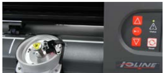
Step 30: Turn the CII on its legs, (without the bottom pan) , plug in the power cord, and turn on. The carriage will move to the right then back to the left, both sorter bowls will have the LED's blink and the wheels will rotate, then a red light followed by a green light on the keypad will show. You have successfully installed the main board.
