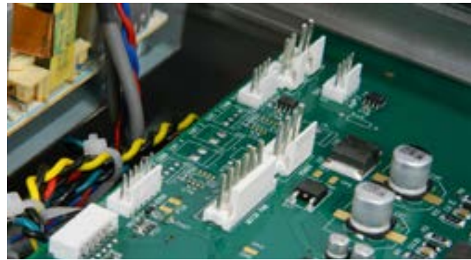
Step 10: All connectors and carriage ribbon on the left side of the board are disconnected.
