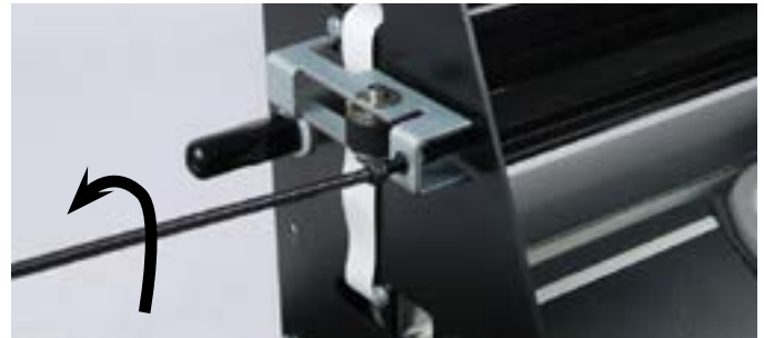
Step 4: With an Allen wrench 11/32", loosen the tensioner screw 2 full turns counter clockwise. This will loosen the Y belt.
