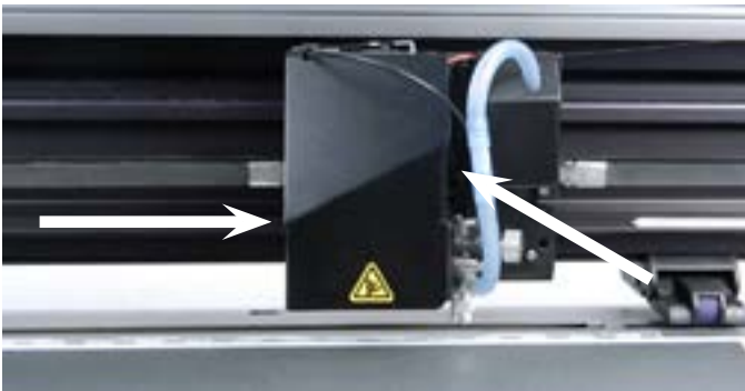
Step 5: Remove the carriage cover by removing the 2 screws as shown by the arrows.
