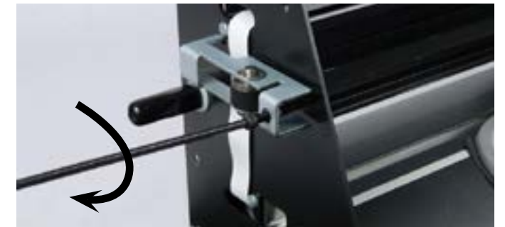
Step 20: With an Allen wrench 11/32", tighten the tensioner screw 2 full turns clockwise. This will re-tighten the Y belt.
