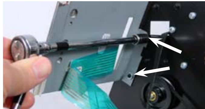
Step 10: Remove the key pad by un-screwing the 2 locking nuts with the 11/32 socket and the long extension.
