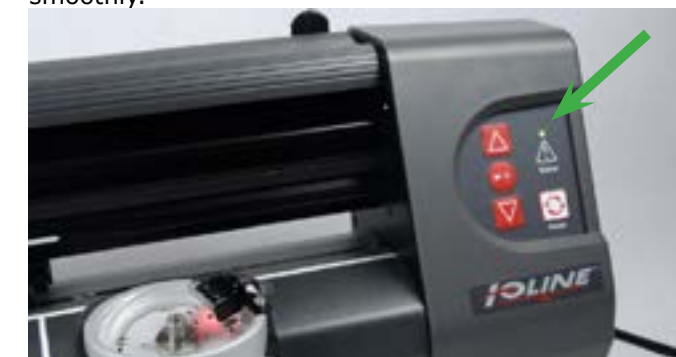
Step 23: When the carriage moves back to the left end plate, a green light should appear on the Status Triangle (green arrow). You have successfully installed the new keypad.
