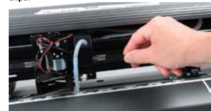
Step 21: Before placing the end covers back on, you need to make sure that the carriage slides left to right smoothly.
