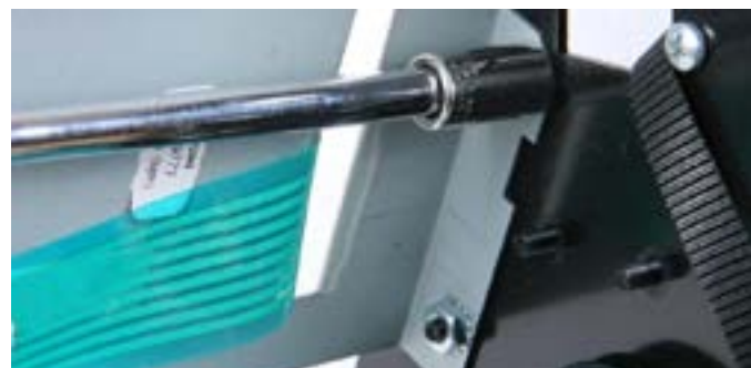
Step 16: Attach the new key pad on the right end plate. Align the holes with the 2 threaded studs and place the locking nuts on by hand, then tighten down with the 11/32 wrench with extension.
