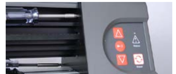
Step 24: You can now place the 2 screws to secure the end cover.
