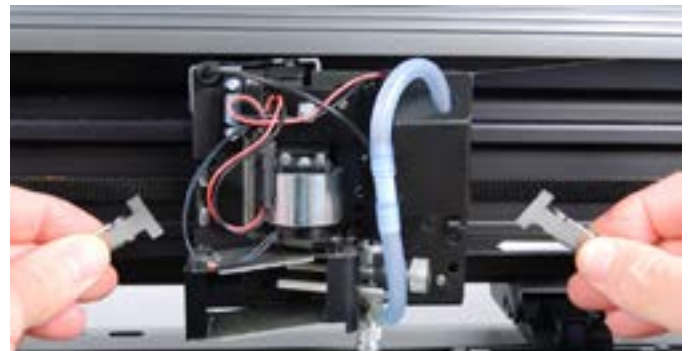
Step 6: Remove the 2 clips from the carriage base plate. This will free up the Y belt for the removal of the Y transmission below in step 8.
