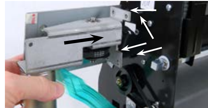
Step 17: Install the Y transmission by placing it over the 4 threaded studs (4 white arrows), then hand tighten the 4 locking nuts.
