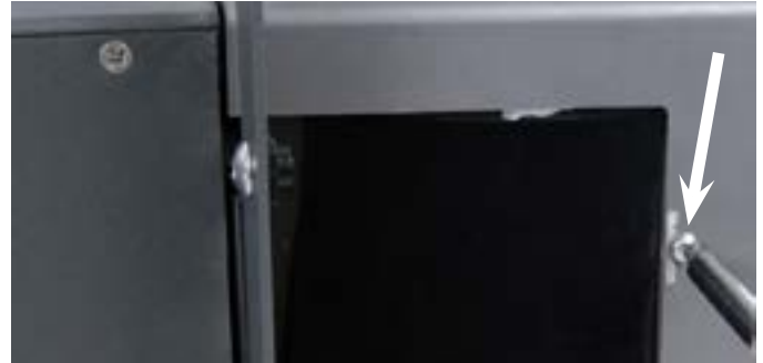
Step 2: Tilt the machine on its back, remove the 1 screw on the bottom of the right end cover, then tilt the machine back up-right. Slide the end cover off the end plate for access for the removal of the keypad.
