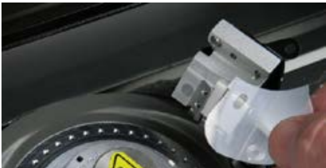
Step 11. Using the notch on the shield as a guide, place the shield as shown and press down onto the tape.
