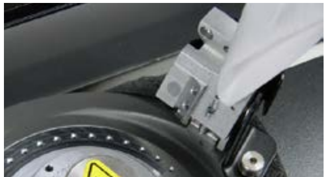
Step 8. Clean area with Alcohol for the placement of the new tape pieces.
