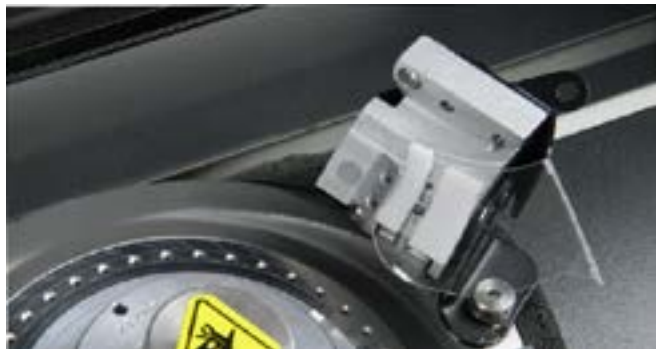
Step 5. An unobstructive view of the shield to be removed.
