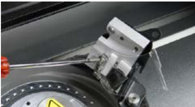
Step 13. Re-install the wiper using the 2 screws. Do NOT over tighten. (Over tightening the screws may damage the wiper)
