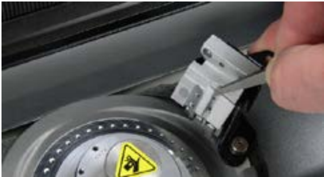
Step 9. Cut new tape to size and adhere.
