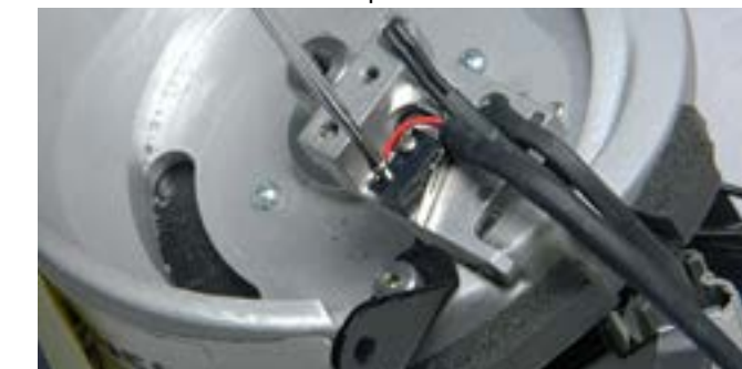
Step 22: With the screws in place, align the screws up with the holes. The holes are threaded and will screw in the metal arm.
