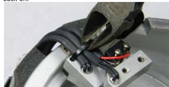
Step 15: With the wires cutters, cut the black tie wrap. IMPORTANT: BE CAREFUL NOT TO CUT THE BLACK WIRES.
