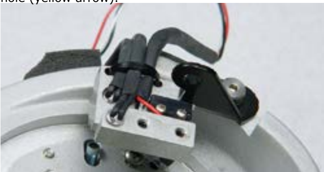
Step 27: The tie wrap should appear as above. Tight over the 3 wires. Place back on, the black metal cover that you see back in step 12.
