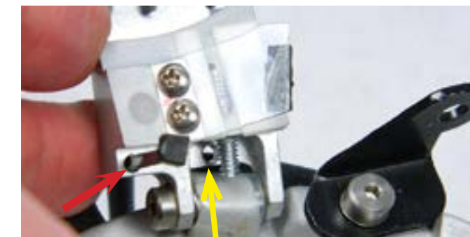
Step 24: You now need to insert the black tie wrap. You start it on the bottom (side as shown, red arrow).
