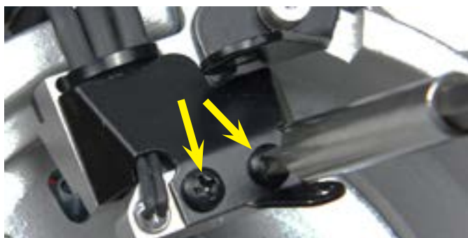
Step 12: With the normal phillips screwdriver, remove the 2 black screws from the cover (arrows).
