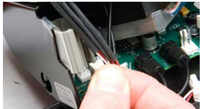
Step 28: With the arm closed and locked (step 27), place the 3 wires back in the grey plastic clip as shown.
