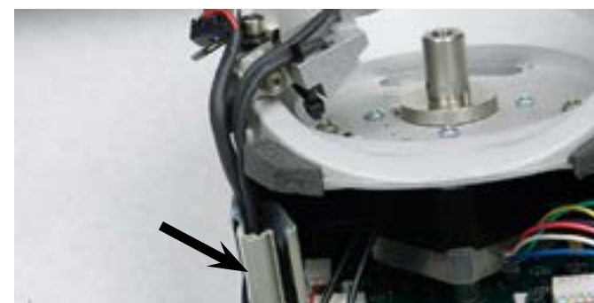
Step 17: You need to unhook (open) the grey plastic cable channel (arrow).
