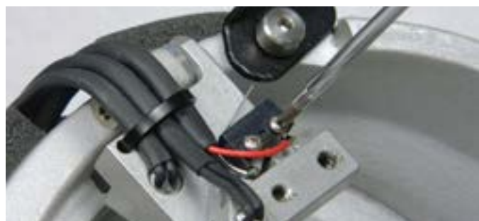
Step 14: With the small phillips screwdriver, unscrew both of the screws that hold the limit switch to the jaw. The screws may remain in the old switch. Just pull them out the rest of the way with a tweezers. NOTE: You will re-use the screws for the new limit switch.
