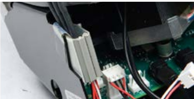
Step 29: Snap close the grey plastic clip to keep the wires in place.
