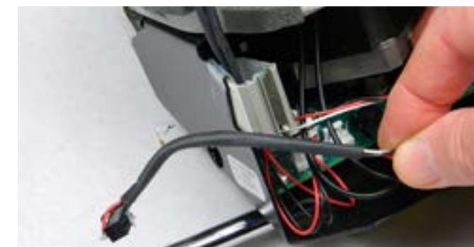
Step 18: Grab the old limit switch and pull it out from the cable channel as shown. NOTE: The other 2 wires remain in the cable channel.
