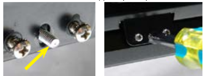
Step 32: Once the bowl is inserted correctly, you should be able to see the threaded stub as in the left photo. Tighten the nylon locking nut until the bowl will not move in or out. Turn the CPII on its back and screw on the 3 nuts and fully tighten, then back off 1/4 turn.
