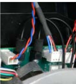
Step 31: (left photo) Re-insert the 2 white clips, (Comm) and the (power). You can now place the bowl back in. The bowl MUST be inserted all the way in. You can view step 7 & 8, or look at the bowl that you did not pull out.
