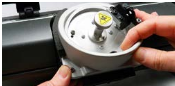
Step 9: Once all 4 locking nuts are removed, you can remove the bowl from the bracket by pulling out about 1 inch, then lift up about 1 inch. You can now pull the bowl out until the 2 wires that connect the bowl to the main board prevent you from pulling further (about 3 inches). See step 10.
