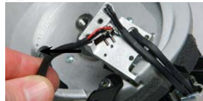
Step 21: With the new limit switch in hand, it will be easier to place the 2 small silver screws in the black plastic portion of the limit switch before screwing onto the jaw, they will slide in.
