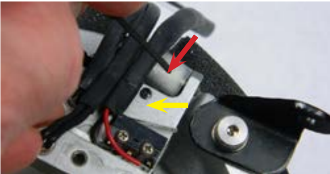
Step 25: The tie wrap, after inserting in the 1st hole, wraps over all 3 wires (red arrow), and enters the 2nd hole (yellow arrow).
