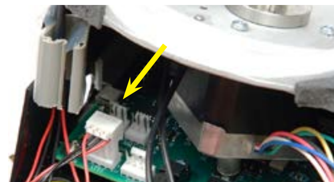
Step 19: Shows the limit switch (arrow) already removed from the board. This is the 'Arm sensor'. It has 3 wires Red, Black and White. Discard the old limit switch.
