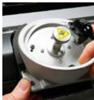
Step 31: (left photo) Re-insert the 2 white clips, (Comm) and the (power). You can now place the bowl back in. The bowl MUST be inserted all the way in. You can view step 7 & 8, or look at the bowl that you did not pull out.
