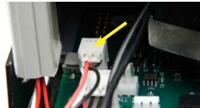
Step 30: Re-insert the limit switch (white clip) into the sorter bowl board. 3 prongs, reads "Arm Sens". Shown on how it should appear (arrow).
