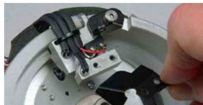
Step 13: Once both screws are removed, lift the cover off and place to the side. You will be placing the cover back on.
