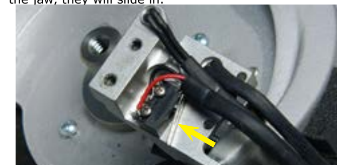
Step 23: IMPORTANT: THE LIMIT SWITCH MUST GO IN THE WAY AS SHOWN. NOTE: THE ARROW POINTS TO THE LEVER.
