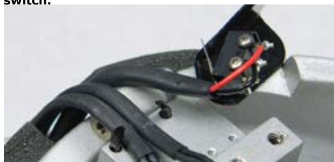
Step 16: The limit switch is now free from the arm. You now need to turn the bowl towards you to view the bowl board. Steps 17, 18 and 19.
