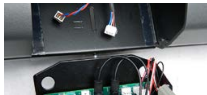
Step 11: This shows the 2 wires un-clipped. You can now move the bowl out to replace the limit switch.
