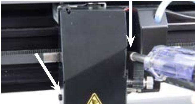
Step 3. Remove the carriage cover. (2 screws).
