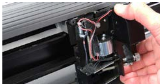
Step 16. You are now ready to place the carriage on the traverse. Make sure the belt is behind the carriage. Push the top of the carriage into the channel between the top cover and the traverse until the top wheel rests on the top rail of the traverse.
