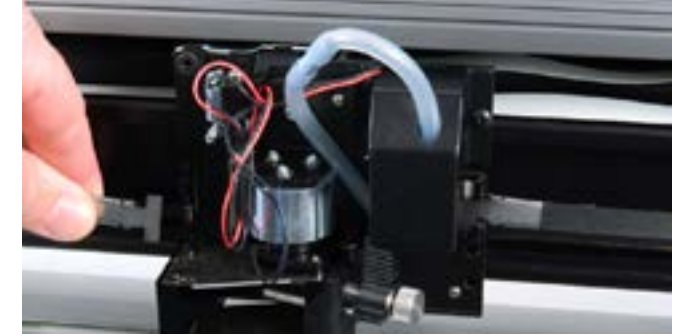
Step 20. Re-attach both belt clips to the carriage as shown above. Hold the carriage with the other hand for stability. NOTE: Check that the belt is NOT twisted.
