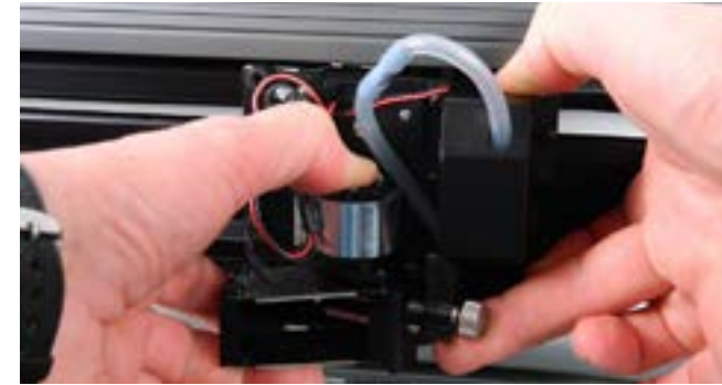
Step 17. Using both hands, press down (spring action) and allow the bottom 2 wheels to go under the bottom rail of the traverse.
