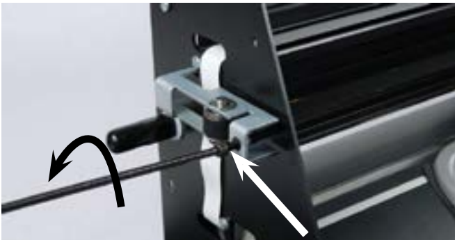
Step 5. With a hex key (9/64), loosen the (Y) carriage belt by turning the tensioner screw 2 full counter clockwise turns. You can use a pliers if you do not have a hex key.
