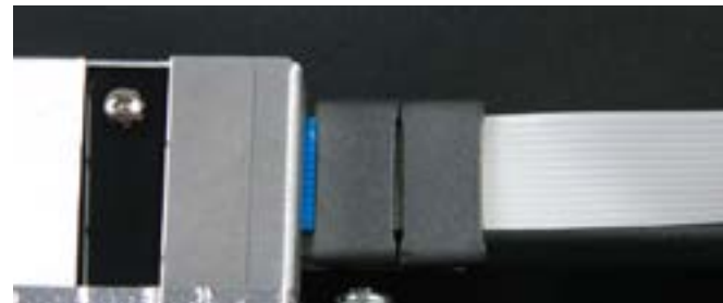
Step 13. With the ribbon cable fully inserted, slide both ferrites in as shown above.
