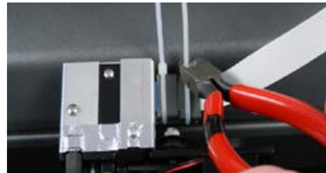
Step 14. Place cable ties around the ferrites and the silver base plate (ties must seat in the notches) then pull tight. You MUST position the nubs and clip off the wraps as shown.
