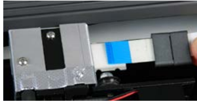
Step 9. Hold the white ribbon cable and gently pull straight out until you see the entire blue section of the cable. Set aside the old carriage (the old carriage will go into the static bag later).
