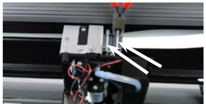
Step 8. With the carriage pulled out to the point shown, cut the 2 cable ties holding the ribbon cable and ferrites. Slide the ferrites back along the ribbon cable. Do NOT remove the ferrites.
