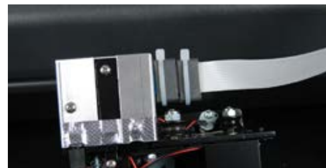
Step 15. Both of the tie wraps have been trimmed. This is exactly how it should appear before you place the carriage on the traverse.
