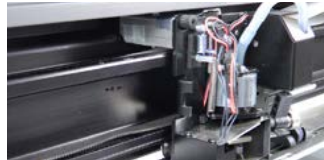
Step 19. This is how the carriage should appear when all 3 wheels are correctly riding on the upper and lower rails. You should be able to slide the carriage smoothly left to right. NOTE: Belt is behind the carriage.
