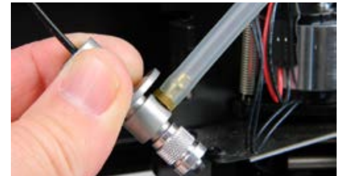
Step 22. The vacuum hose should be pressed all the way in as shown.
