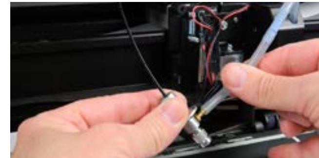
Step 21. Place the vacuum tube onto the brass fitting of the C-stick securely. (Press all the way on).
