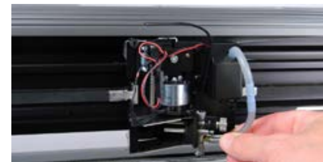
Step 23. Place the C-stick into the jaw, close the clamp, and tighten the thumbscrew. NOTE: Make sure that the clamp is securely holding the C-stick body in the jaw.
