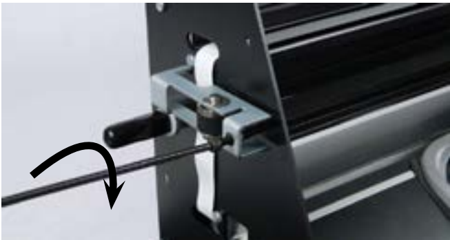
Step 27. Tighten the Y belt at the tensioner by turning 2 full turns clockwise.
