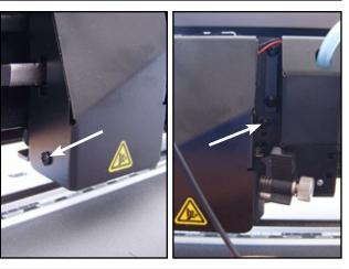
Carefully remove the cover from the carriage and set aside.
