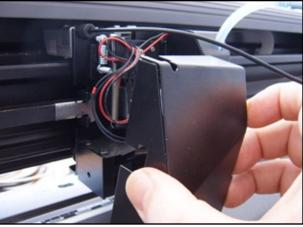
Re-installation is the reverse of the removal steps. Make sure not to pinch any wires in the cover before tightening the screws.
